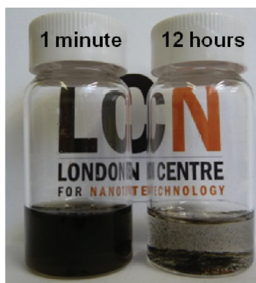
Figure 6. Spontaneously dissolved fraction from a 1:10 metal to carbon ratio reduction stored in inert atmosphere for 6 months, 1 min and 12 h after exposure to air.
